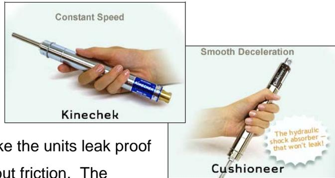
The high-pressure cylinder used in these products is hardened and honed to a mirror finish and individually mated to its piston within a clearance of nominally .0005 inch. This metal-to-metal fit eliminates the need for a sliding piston seal, which provides a greater capacity for its size and an extremely long service life due to no sliding seal wear.
