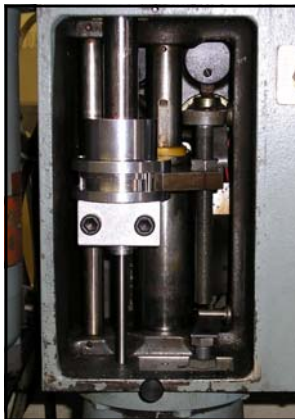
After —with new Slimline kit installed. Adaptor plus 100x-31-x Slimline Kinechek installed.
